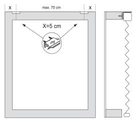
The headrail shall not be installed less than 1,5 m from the floor, and the cord cleats shall be installed as close to the headrail as possible and in all cases, not less than 1,5 m from the floor.
